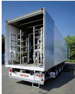
2 x Double Pass RO 2 x 25000 L / H build in a container
